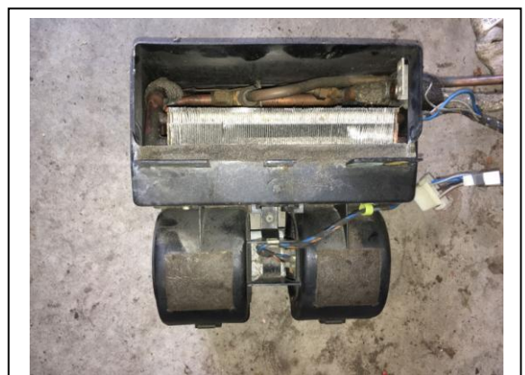
On most vintage cars with A/C, you’ll find an evaporator assembly housing the evaporator core, expansion valve, and blower fan inside the center console.
