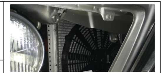
Compressor to left Condenser with cooling fan to right
