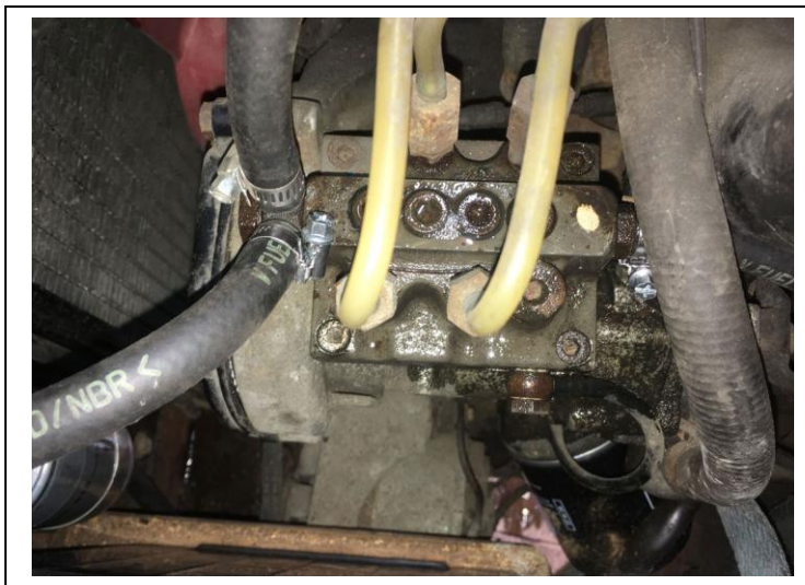
Leaking o-rings in the injection pump of a BMW 2002tii
